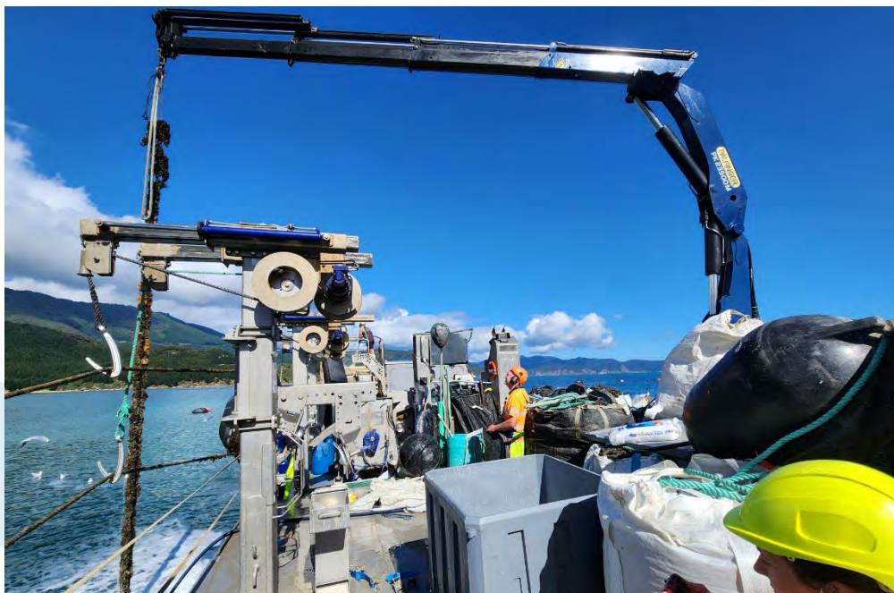
Mussel droppers being picked up and craned straight into a salt slurry within a Dolav™ on the deck of the MacLab vessel, 'Vanguard', during treatment trials.
