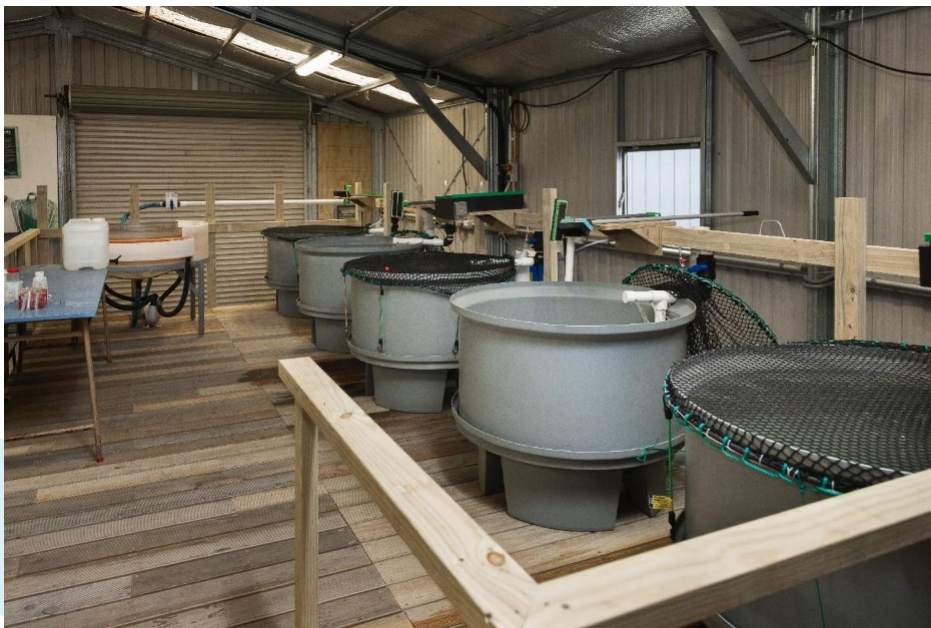
Recent upgrades to the wet lab include a small-scale Recirculating Aquaculture System or 'RAS'
