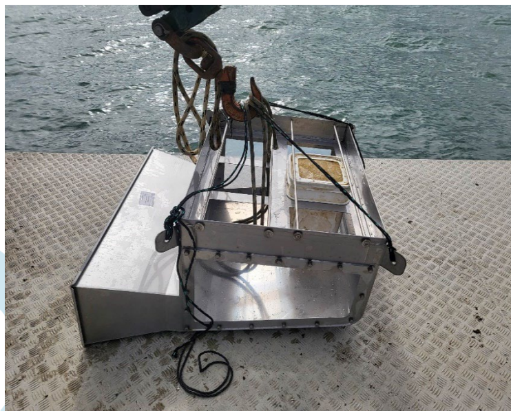
Fig. 3. Photograph of a modular tidal FLUPSY based on previous designs that was tested at a spat farm in Aotea Harbour.
