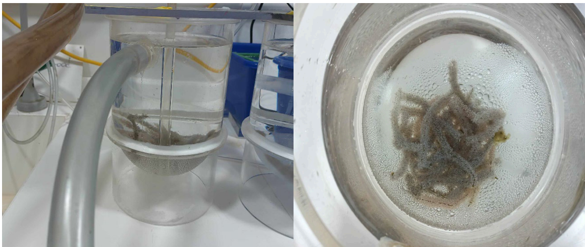
New and improved octopus embryo incubation system where octopus egg strings are loosely placed inside, and a gentle water stream generates a continuous tumbling of the egg strings.
