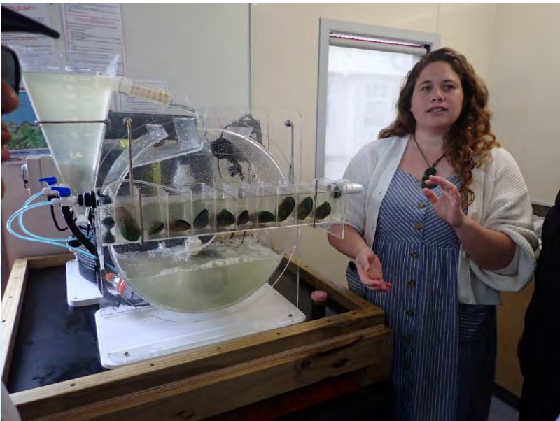
Heni Unwin, Cawthron Māori researcher in marine technologies, demonstrates the shellfish experimental station as part of Ahumoana Whakahihiiko, the first offering of Cawthron's 'Inspiring Aquaculture' programme at Ōpōtiki College. The recirculating system specially built by Cawthron engineers and shipped to the school will help students study mussel feeding, respiration and behaviour as part of their NCEA studies at the college in 2024 and beyond.
