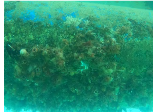
Example of biofouling on a yacht keel where Mediterranean fanworm is present. (Photo by Boffa Miskell)
