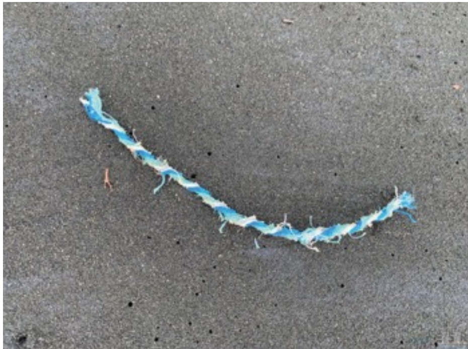
Polymer twine found on the strand line showing evidence of extreme weathering.
