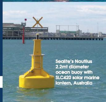
Sealite's Nautilus 2.2m diameter ocean buoy with SLC420 solar marine lantern, Australia
