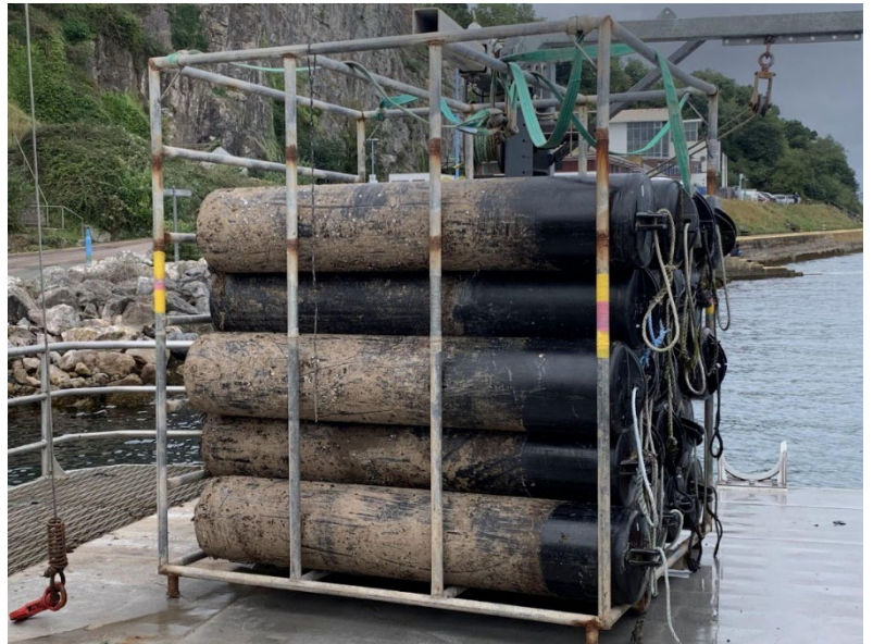
Figure 3. A crate of spar buoys fitted with proprietary end caps on the deck of the Holly Mai. Marine growth shows the typical depth of submergence.
