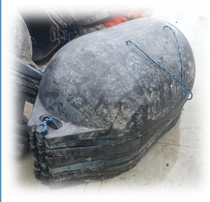
Clean float by scraping (or waterblasting) & cut in half.
