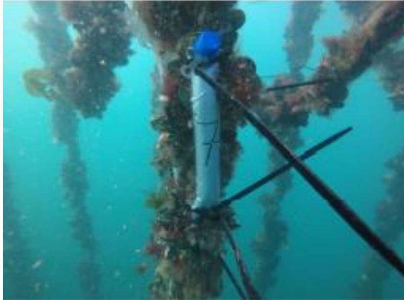
**Figure 3-4: Semi-permeable membrane bag attached to a mussel dropper.** This study was undertaken at a farm in Homewood Bay, Pelorus Sound. NIWA is grateful to Sanford Ltd. - who gave us access to their farm and provided logistical support for the study.
